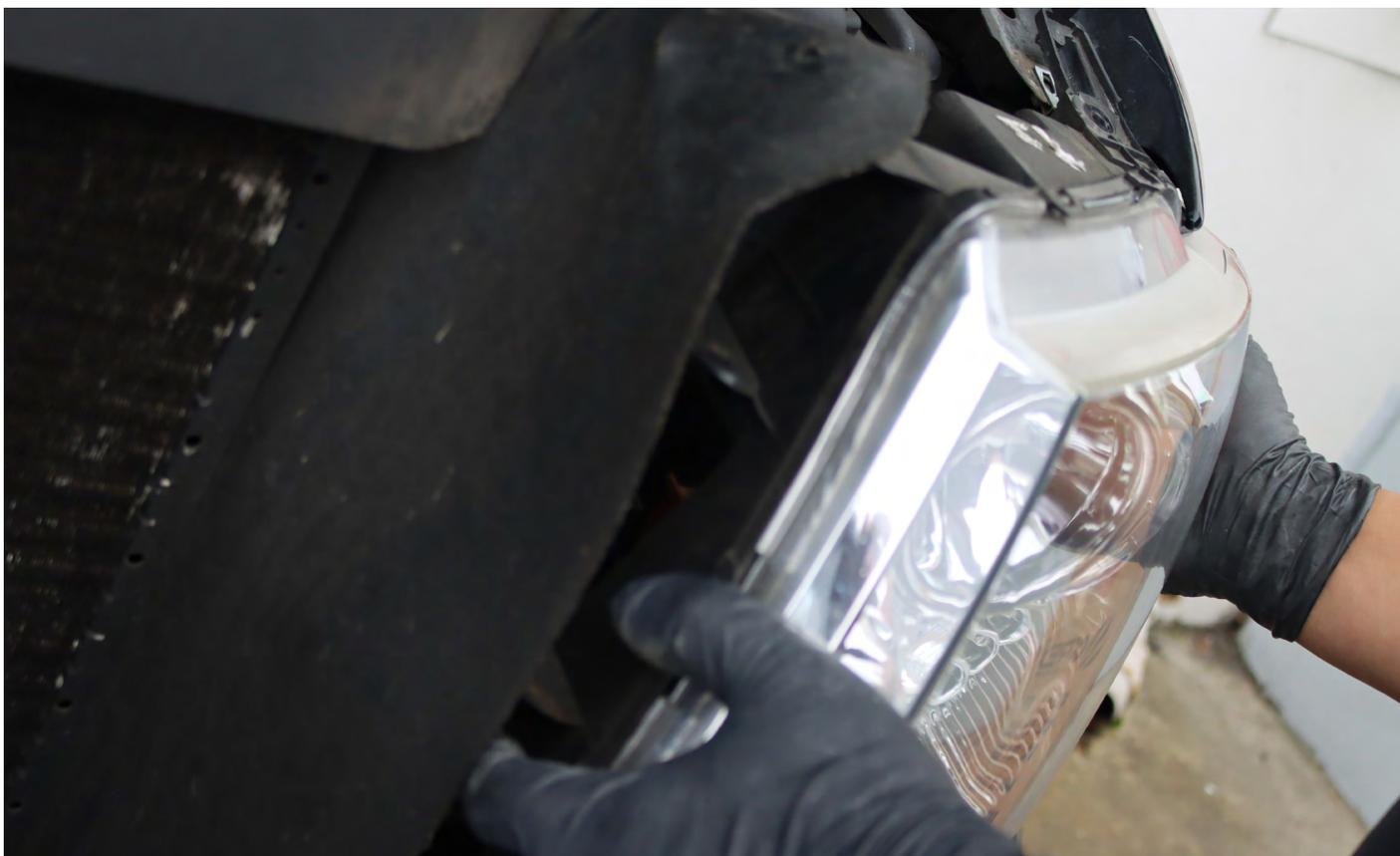
Disconnect the sockets and take out the parking light bulb from each side of the headlight.
