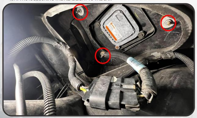
13. REMOVE THE SIX T15 TORX SCREWS FROM THE TOP EDGE OF THE FENDER, AND THE ONE 10MM NUT FROM THE BOTTOM OF THE FENDER BY THE HEADLIGHT. THIS WILL ALLOW THE FENDER TO BE MOVED SLIGHTLY TO ALLOW THE HEADLIGHT TO BE REMOVED
