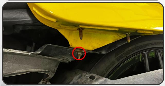
14. WITH THE FENDER UNBOLTED, GENTLY FLEX THE FENDER UPWARDS AND OUTWARDS ENOUGH TO LIFT THE HEADLIGHT UP AND OUT OF THE HEADLIGHT CAVITY. BE CAREFUL NOT TO FLEX THE FENDER TOO MUCH AND CRACK THE FIBERGLASS, BUT THE FENDER WILL BE ABLE TO MOVE ENOUGH FOR THE HEADLIGHT TO CLEAR THE OPENING
