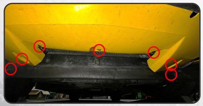
11. OPEN THE HOOD OF THE CAR. REMOVE THE FOUR T15 TORX SCREWS FROM THE TOP EDGE OF THE HOOD. WITH THE BUMPER NOW FULLY UNBOLTED FROM THE CAR, LIFT UPON THE TOP EDGE BY THE HOOD, AND THEN PULL THE BUMPER FROM THE CAR
