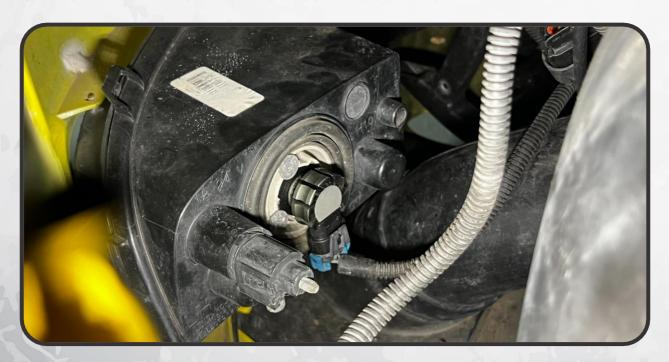
8. REMOVE THE TWO 10MM NUTS SECURING THE SIDE OF THE BUMPER TO THE FENDER
