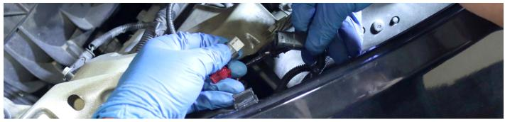
Proceed by attaching the converter connector to the ALPHAREX headlight unit, and then connect it to the vehicle's lights connection DO NOT USE DIELECTRIC GREASE!
