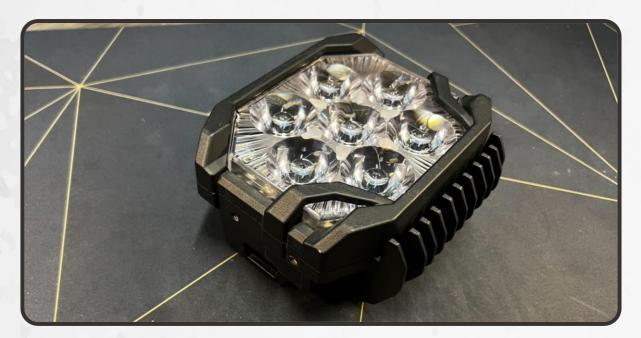
7. FLIP THE POD BACK OVER ONTO ITS FACE. WE RECOMMEND TAKING THIS TIME TO ADD A DROP OF THREAD LOCKER TO THE THREADS OF EACH OF THE SCREWS. REINSTALL THE 4 SCREWS INTO THE POD AND TIGHTEN THEM DOWN IN A STAR PATTERN UNTIL HAND TIGHT
